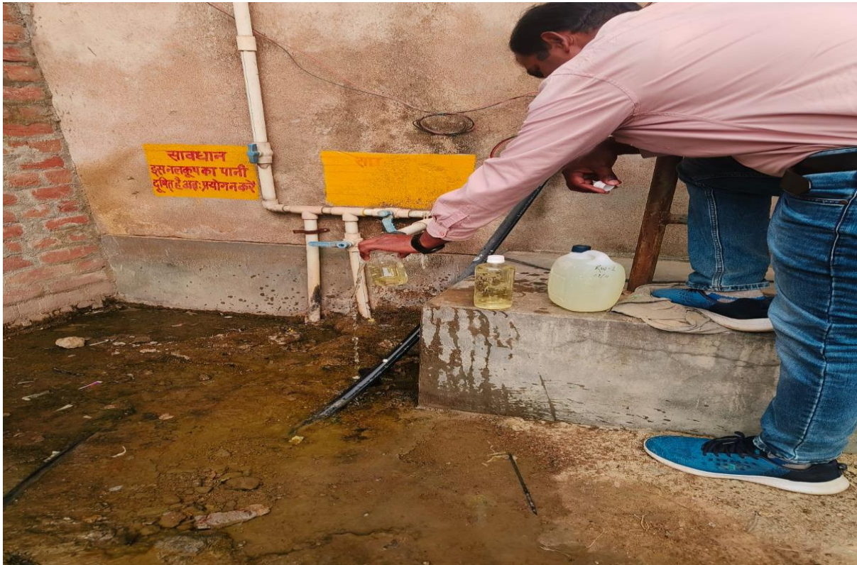
Image 27: Borewell water sampling (green color groundwater) from nearby unit
